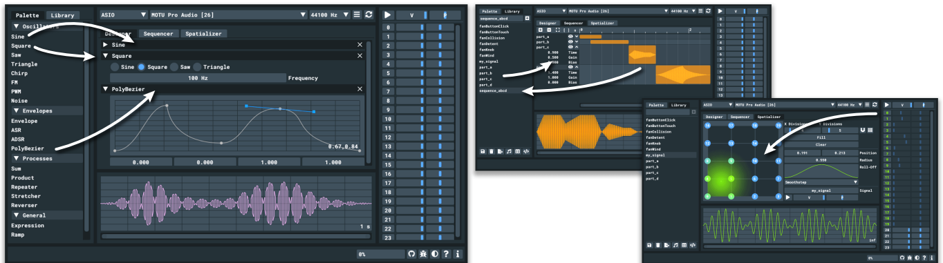
Figure 8: Syntacts GUI - The left-hand side demonstrates cue design. Users drag, drop, and configure Signals from the design Palette to the Designer workspace. The Signal is visualized and can be played on individual channels of the opened device. The right-hand side shows the GUI’s track-based sequencer (background) and spatializer (foreground) interfaces. Once designs are complete, they can be saved and later loaded from the programming APIs.
