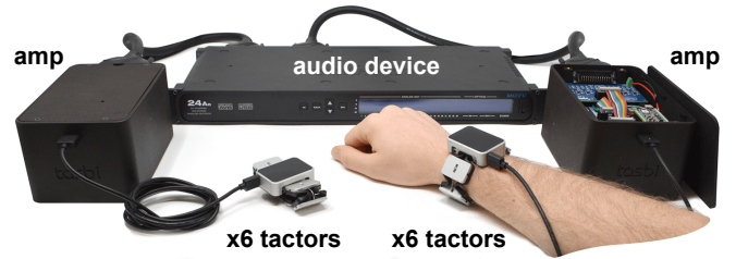
Figure 9: Syntacts In Use - This figure demonstrates a real-world implementation of the Syntacts amplifier, where it has been used to drive two Tasbi haptic bracelets [3]. A professional grade audio device (MOTU 24A0) is connected to two Syntacts amplifier boards that have been integrated into separate Tasbi control units. Amplifier output is transmitted to each Tasbi over a multi-conductor cable. Each Tasbi bracelet incorporates six Mplus 1040W LRA factors radially spaced around the wrist, for a total of twelve utilized audio channels. The audio device interfaces with a host PC (not shown) through a USB connection.
