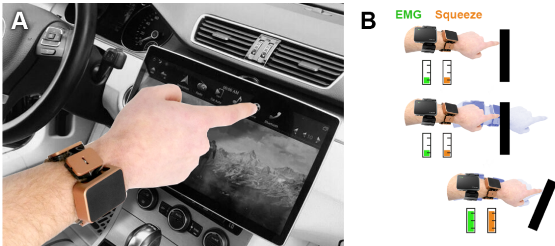
Figure 9.2 : Integrating Tasbi with other technologies presents interesting opportunities. (a) Devices like Tasbi can provide haptic feedback for ordinary capacitive displays. (b) Emerging technologies, such as brain-machine interfaces and electromyography (EMG) might enhance the believability of Tasbi-mediated interactions in XR.
