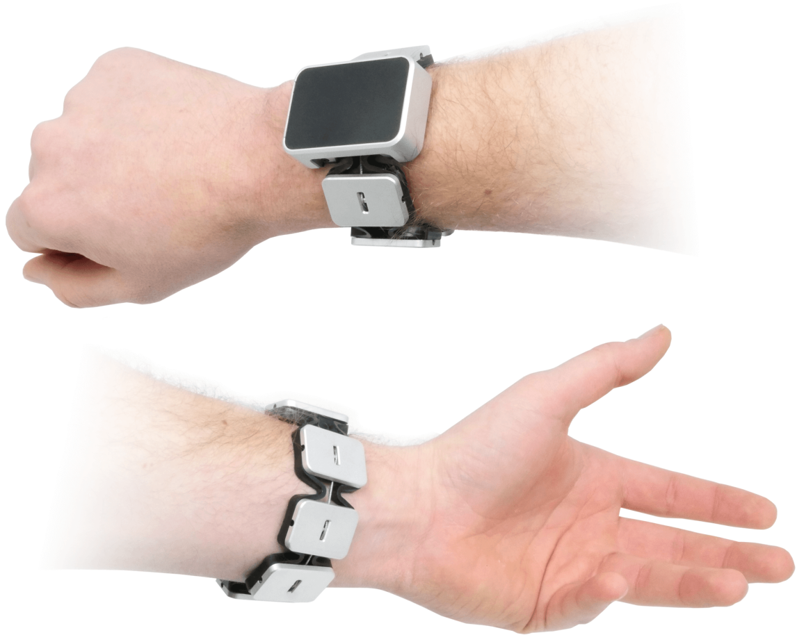
Figure 3.1 : The final iteration of Tasbi as worn on the wrist. The device incorporates six vibrotactile actuators and a novel squeezing mechanism. Not pictured is the tethering cable required to power and with interface.
