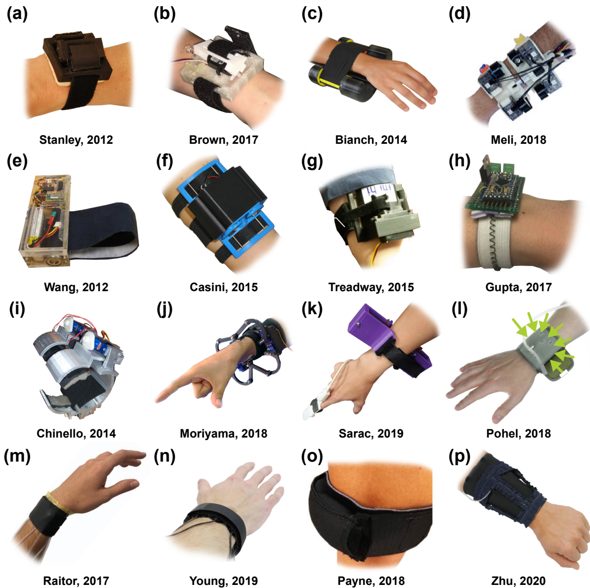
Figure 2.2 : Squeeze Bracelets and Armbands — (a-g) Electromechanical, band-based devices. (h) A device employing shape memory alloys. (i-k) Devices that squeeze only in the normal direction. (l-p) Pneumatic based squeezing devices.
